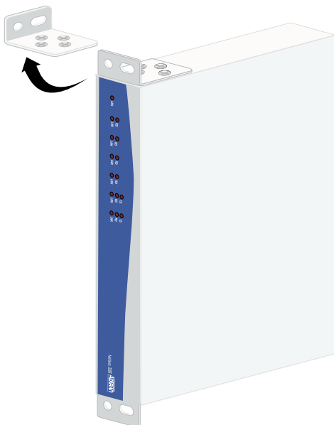
Figure 16. Repositioning the Mounting Bracket
