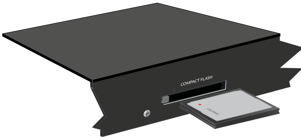
Figure 20. CompactFlash Card Installation
