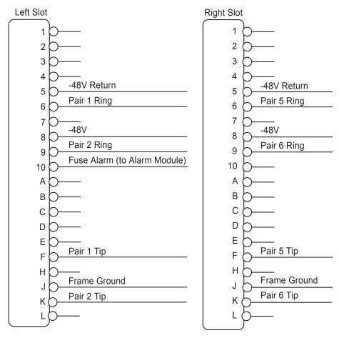
NOTE: Connect only those output pairs required to meet power requirements of the Total Access 1124 DSLAM based on the transmission distance.
