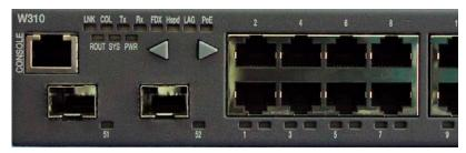
Connect the Console cable to the W310 Console port. (Step 2)
