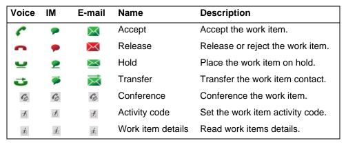
Only appropriate controls are displayed on work items. Voice-related controls are displayed on a voice work item. IM related controls are displayed on IM work item.
