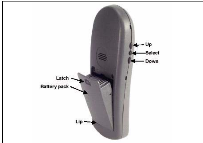
Figure 5 WLAN Handset battery pack location
