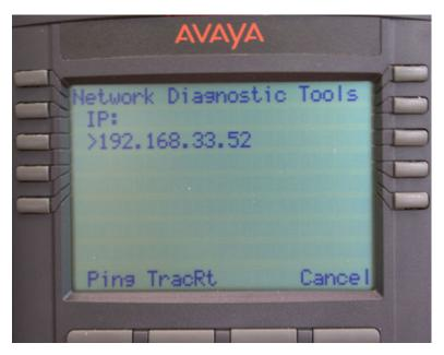
Figure 79: Network Diagnostic Tools screen
