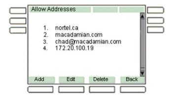
Figure 74: Allow Addresses screen with domains and SIP addresses
