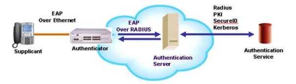
Figure 39: 802.1x and EAP network architecture
