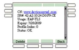
Figure 33: Device Certificate details
