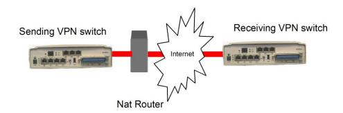
The BCM50 Integrated Router solves this problem by the use of NAT Traversal; an option that can be selected when configuring VPN Branch rules. Both VPN switches should have NAT Traversal enabled.
