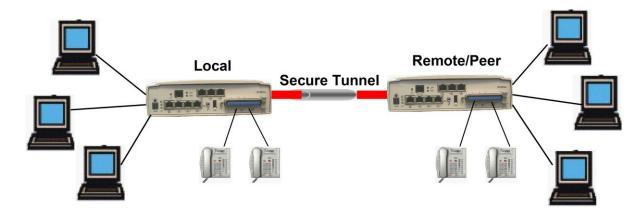
When configuring Branch rules, settings must be agreed upon before configuration can successfully take place. These settings include security details (IKE, VPN Protocol, Pre-Shared Key), and manually entered information such as WAN IP Addresses, Local/Remote IP Addresses, Content Type etc. The information must match on both the local and remote ends otherwise the connection will not be successfully made.
