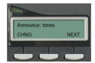
5. The Announcements option appears showing the current setting. Press CHNG to change this setting. Each time you press CHNG, the setting changes to one of 'tones', 'names', and 'off'. Press OK to keep the current setting and exit.
