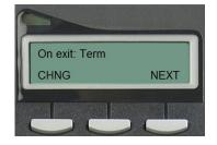
4. The Conference Continuation option appears showing the current setting. Press CHNG to change this setting. This option switches between 'Term' and 'Cont'. Press \* to keep the current setting and exit.
