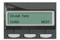
4. The Conference Continuation option appears showing the current setting. Press CHNG to change this setting. This option switches between 'Term' and 'Cont'. Press NEXT to keep the current setting and go to the next option.
