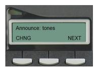
The Announcements option appears showing the current setting. Press CHNG to change this setting. Each time you press CHNG, the setting changes to one of 'tones', 'names', and 'off'. Press OK to keep the current setting and exit.
