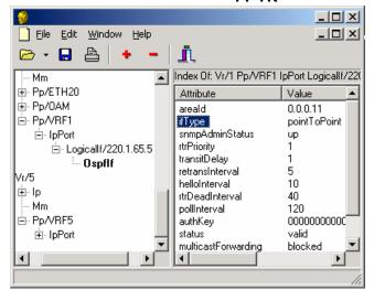
Upon debugging it was found that the PP7k set the value of the iftype parameter to broadcast on all the protocol ports. The Cisco router, on the other hand sets it PointToPoint. If the iftype value does not match the routes do not get populated. Once the iftype on the PP7K was changed to pointToPoint the routes were populated in the routing database.
