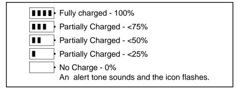
When the batteries are replaced, the battery status does not appear on the display screen until the replaced batteries are charged.
