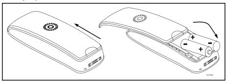
Slide the back cover of the handset upwards to insert or remove batteries.
