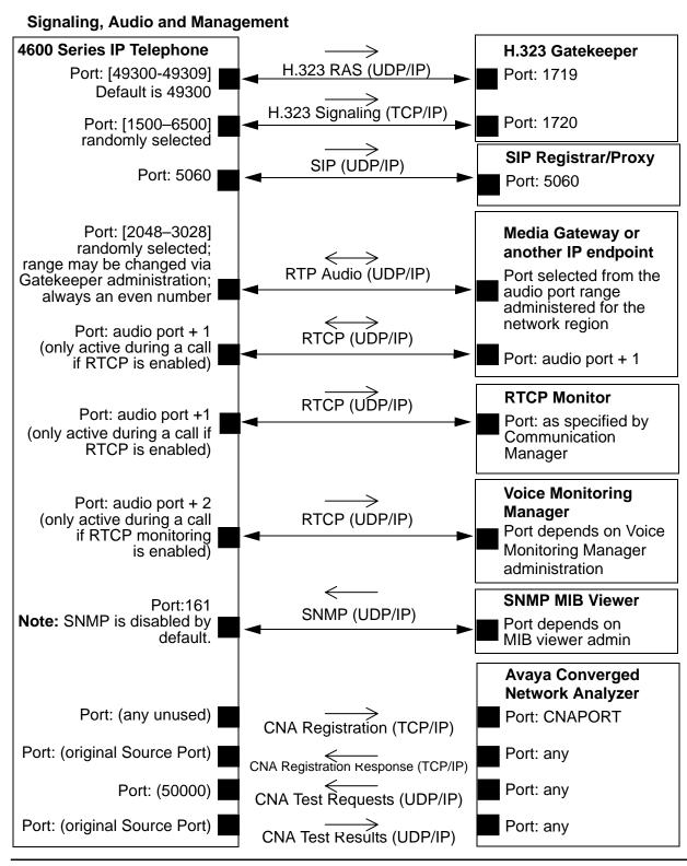
Figure 1: Signaling, Audio and Management Diagram
