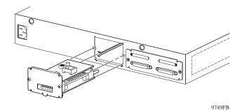
Press firmly to make sure that the DC-DC converter module is fully seated.
