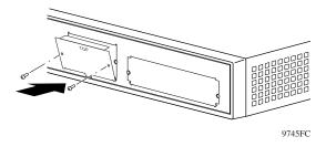
**b** If you have a plate with a domed flange, fit the bottom into the opening and firmly push in the top. Insert the screws and tighten using a Phillips screwdriver.
