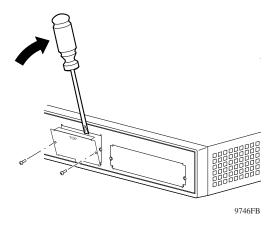
Set aside the blank plate and the screws. If you remove the DC-DC converter module for any reason, be sure to re-insert the blank plate.
