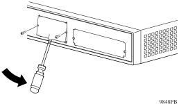
Set aside the blank plate and the screws. If you remove the DC-DC converter module for any reason, be sure to reinsert the blank plate.
