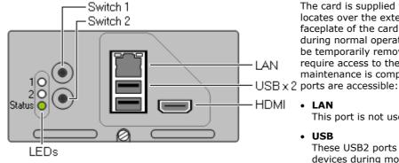
The card is supplied with a removable plastic cover that locates over the external ports (LAN, USB and HDMI) on the faceplate of the card. This cover should always be in place during normal operation of the card. The cover should only be temporarily removed during maintenance actions that require access to the ports and should be replaced when the maintenance is completed. Whilst removed, the following
