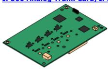
These cards allow the base card to support 4 analog loop-start trunks.
