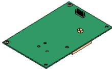
This card allows the base card to support up to 2 PRI trunk connections. The card is available in single and dual port variants. The card can be configured for E1 PRI, T1 robbed bit, T1 PRI or E1R2 PRI trunks.
