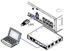
During installation it is recommended that the IP Office control unit is started without it being connected to any network. That ensure that the IP Office defaults to a known set of IP address settings.
