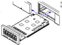
The IP500 base cards and trunk daughter cards should be fitted before power is applied to the control unit.
