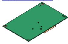
This card allows the base card to support up to 4 BRI trunk connections, each trunk providing 2B+D digital channels. The card is available in 2 port (4 channels) and 4 port (8 channels) variants.
