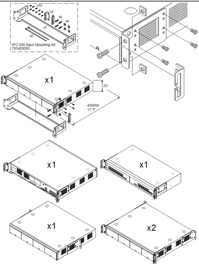
ullet Only the screws provided with the mounting kit should used to attach the brackets to the control unit.
