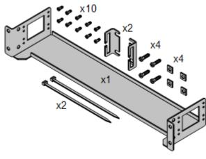
The IP500 control unit and IP500 external expansion units can be rack mounted if required into 19-inch rack systems. This requires an IPO IP500 RACK MNTG KIT (SAP 700429202) for each unit.
