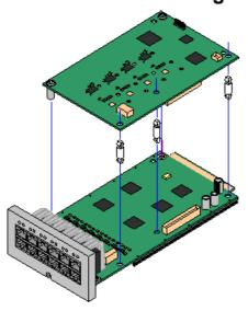
Most <u>IP500 base cards</u> 23 can be fitted with an IP500 trunk daughter cards to support the connection of trunks to the base card.
