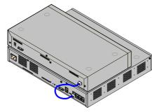
External expansion modules connect to the IP Office control unit using an expansion interconnect cable.
