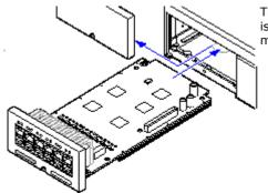
The IP500 base cards and trunk daughter cards should be fitted before power is applied to the control unit. Ensure that cards are inserted in the order that matches the planned or pre-built configuration.
