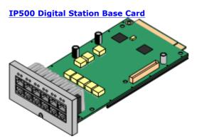
This card has 12 RJ45 ports. The first 8 ports are  $\underline{\text{DS}}$  ports for the connection of Avaya digital phones other than IP phones. The card can be fitted with an IP500 daughter card which then uses the additional 4 RJ45 ports for connections.
