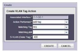
Create an action to add a tag (VLAN 400) to all traffic based on the P-bit for the associated interface.
