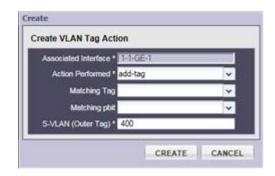
Create an action to add a second tag (VLAN 400) to all VLAN 401 traffic on the associated interface.
