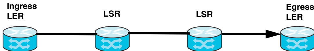
Figure 2-22 Sample static unidirectional tunnel
