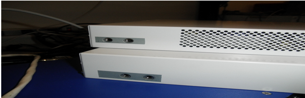
Figure 9-1 Left side of the 3903 chassis, grounding screw location
