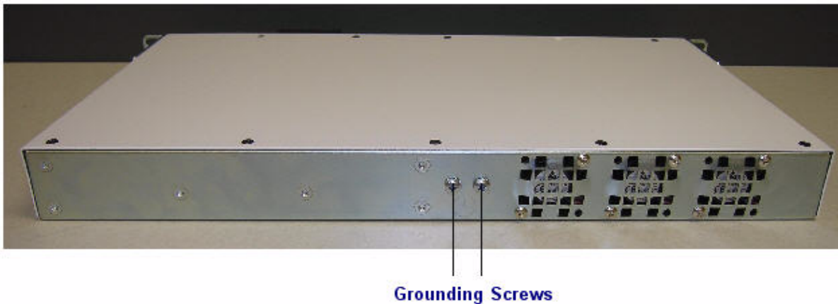
Figure 9-10 Grounding screw location on 5160 switch
