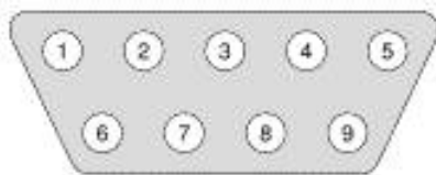
Figure 4-1 DB-9 connector pin-out
