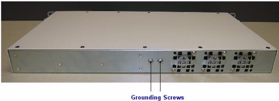
Figure 9-9 Rear grounding screw location
