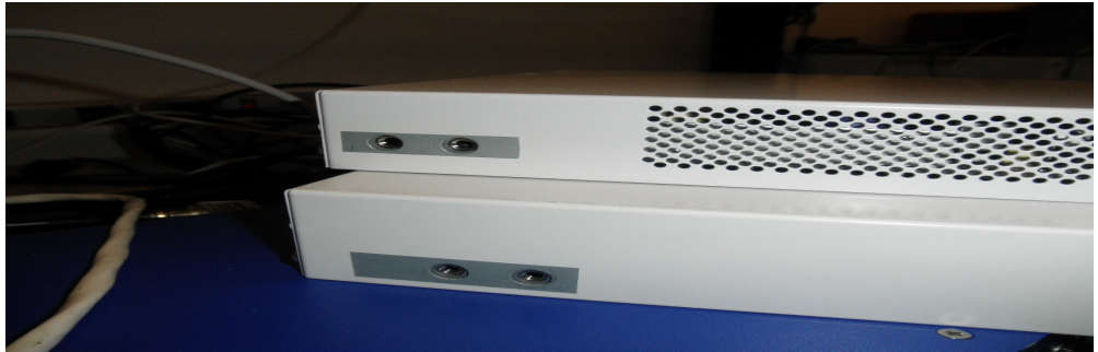
Figure 9-2 Left side of the 3903x chassis, grounding screw location
