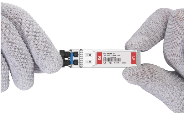
Figure 21: Installing a Protective Cap
