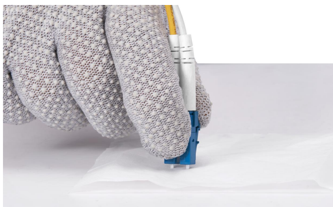
Figure 20: Cleaning Optical Fibers with Special Cleaning Tissues
