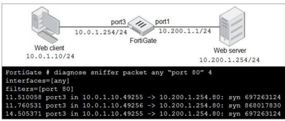
In the network shown in the exhibit, the web client cannot connect to the HTTP web server. The administrator runs the FortiGate built-in sniffer and gets the output as shown in the exhibit.
