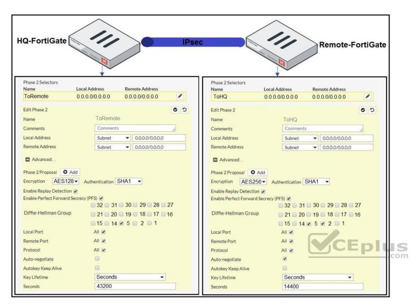
A network administrator is troubleshooting an IPsec tunnel between two FortiGate devices. The administrator has determined that phase 1 status is up, but phase 2 fails to come up.
