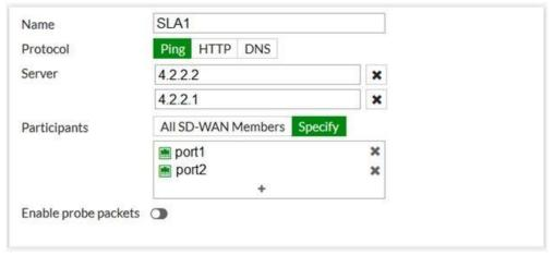
An administrator has configured a performance SLA on FortiGate, which failed to generate any traffic.
