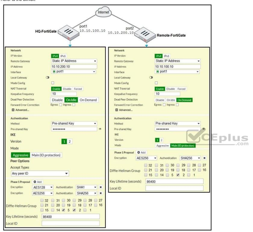
A network administrator is troubleshooting an IPsec tunnel between two FortiGate devices. The administrator has determined that phase 1 fails to come up. The administrator has also re-entered the pre-shared key on both FortiGate devices to make sure they match.
