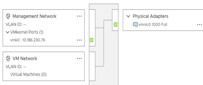
Figure 68: Topology Diagram of a vSphere Standard Switch
