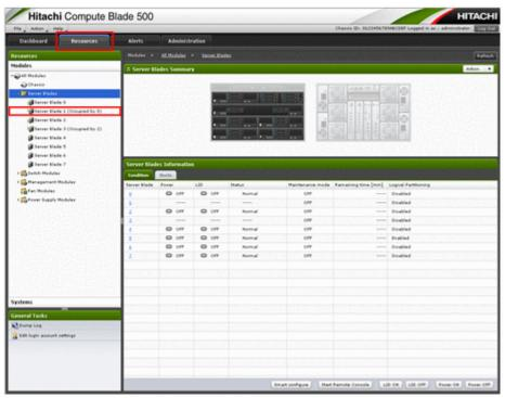
4. Select a target server blade, and click the **Condition** tab. Confirm that the **Logical Partitioning** is **Disabled**, and click **Power ON**.
