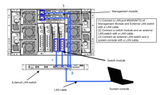
When using the LAN pass through module, the LAN pass through module should be connected to the external LAN switch cable as follows.
