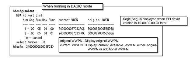
The WWPN is added into the command prompt by executing the "select" command, and you can confirm the target adapter.
