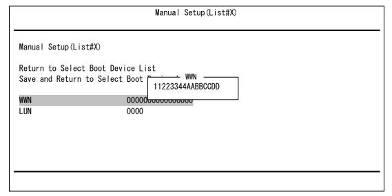
If a character string is inputted and the Enter key is pressed, a dialog will disappear and the setup value of WWN will be changed into "11223344AABBCCDD.".
