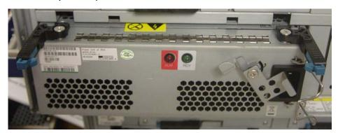
Figure 4-14: Expansion Unit Power Supply Partly Removed Table 4-9: Expansion Unit Power Supply Partly Removed
