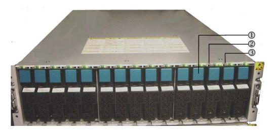
Figure 1-13: Expansion Unit Front View, Bezel Removed
