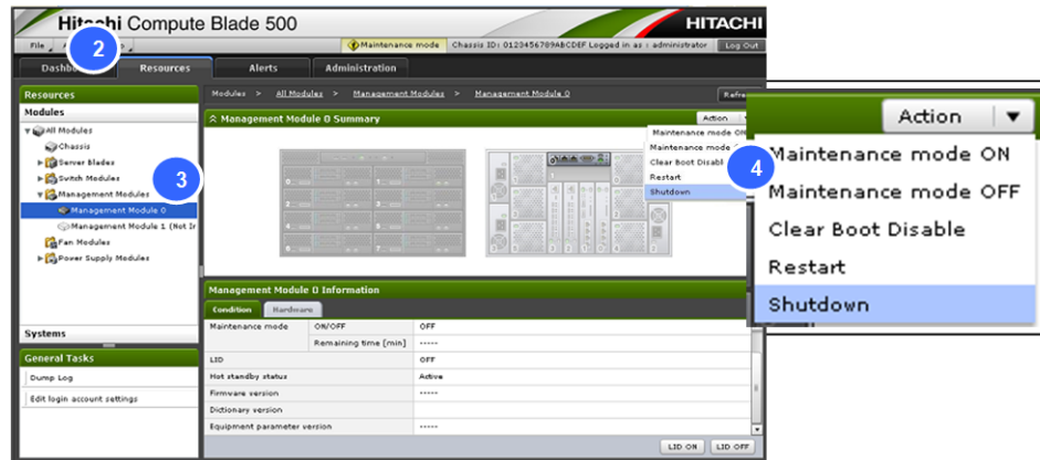
Figure 4-53 Power off procedure of failed management module
