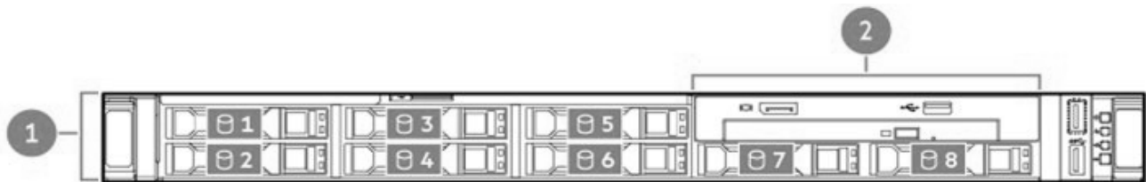
8 SFF+ ODD device bay (optional through Media Bay)
