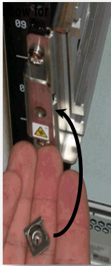
Third nut slides in to lock the tray in place
