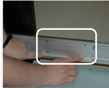
Tighten these four screws on each rail when the rail is in place
