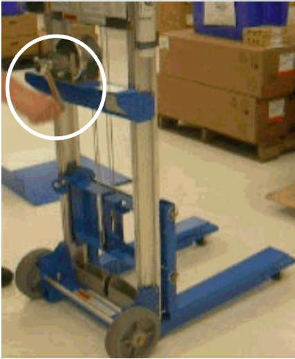
Crank handle for lifting
