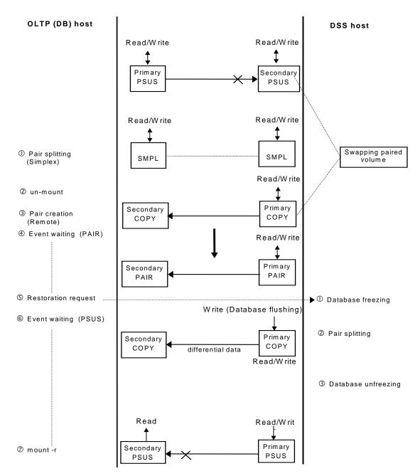
Figure 2-12: Restoring S-VOL to P-VOL in Split Status using ShadowImage
