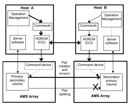
Figure 2-8: TrueCopy/TCE Remote System Configuration
