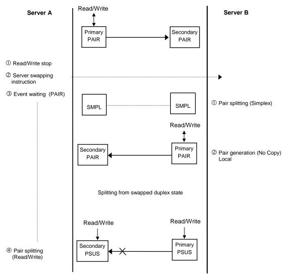
Figure 2-15: Swapping Paired Volume for Duplex Operation Using TrueCopy/TCE
