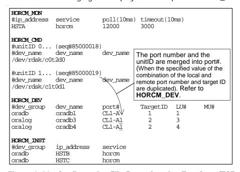
Figure 2-20: Configuration File Example using TrueCopy/TCE – UNIX® - Based Hosts
