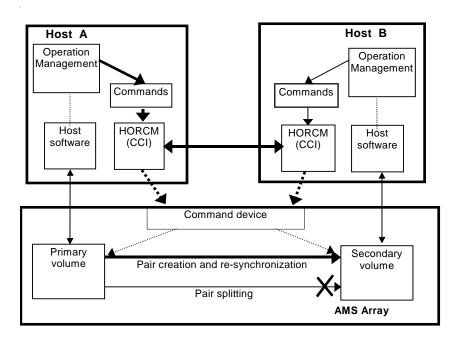
Figure 2-5: SnapShot System Configuration
