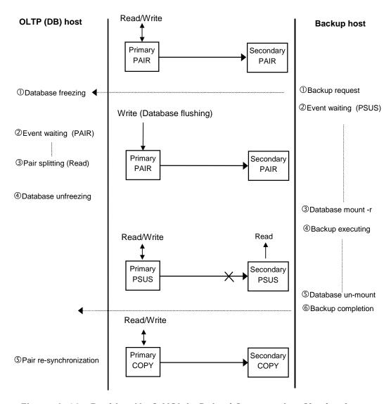
Figure 2-10: Backing Up S-VOL in Paired Status using ShadowImage
