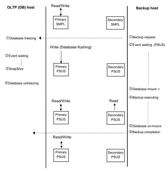
Figure 2-14: Backing Up Secondary Volume (V-VOL)
