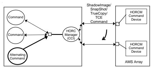
Figure 2-25: Alternate Command Device Function
