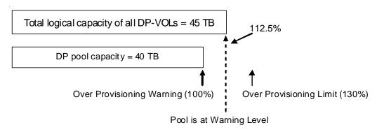
Figure 2-5: DP Pool Capacity when Over-provisioning Warning Threshold Value is 100%
