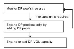
Figure 5-1: Dynamic Provisioning Work Flow
