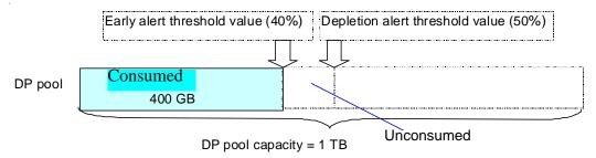
Figure 2-4: DP Pool Capacity If Early Alert Threshold Value is 40%
