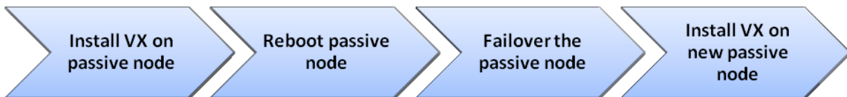
Figure 4: Sequence for Up-gradation in Microsoft Cluster Environment
