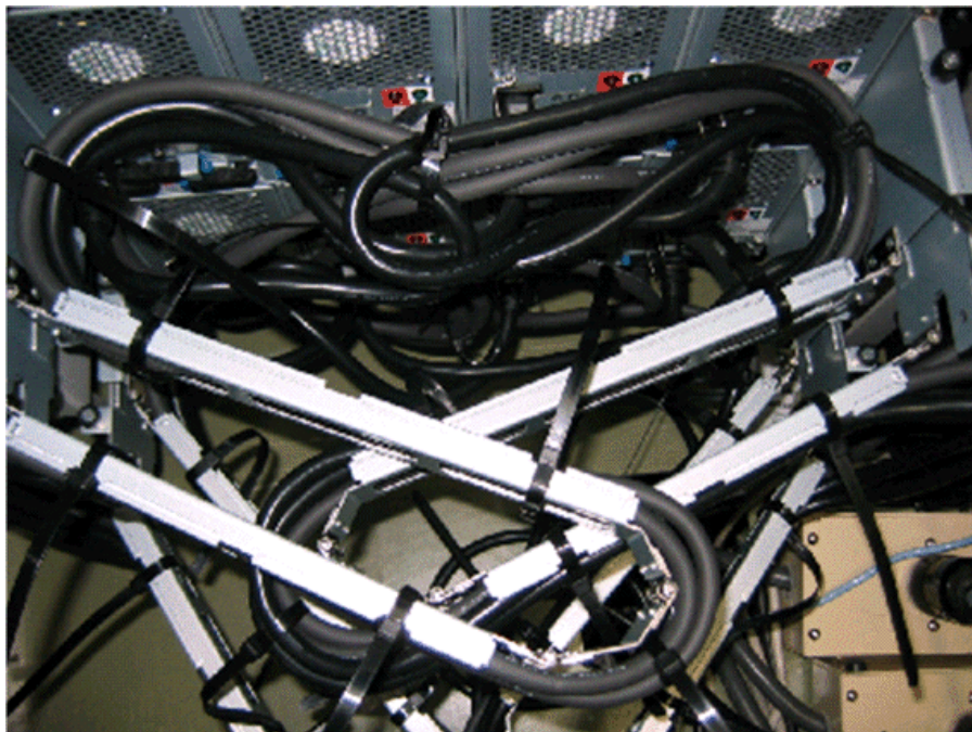
Figure 5-32: ENC Cable Routing on High-density Expansion Unit
