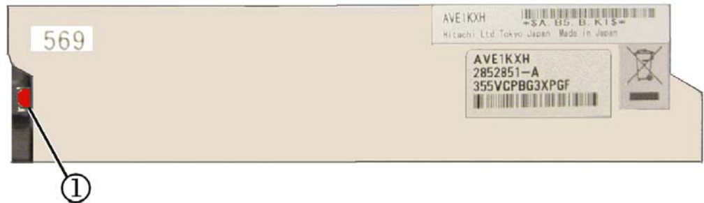
Figure 4-29: Disk Drive Alarm LED
