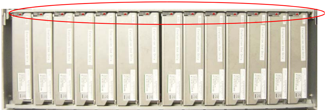
Figure 4-30: Alarm LED Locations
