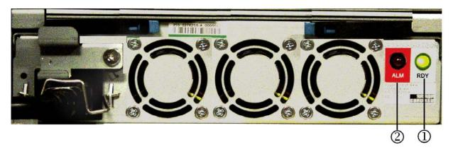
Figure 4-10: Base Unit AC Power Supply LEDs
