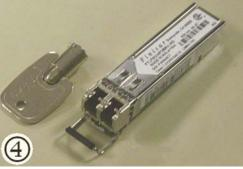
Figure 4-8: Fibre Channel Host Connectors
