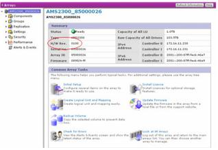
Figure 10-5: AMS 2300 Arrays Screen with 0100 Hardware Revision
