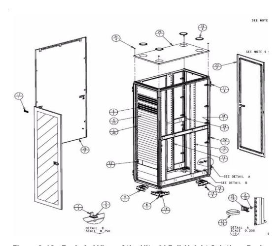
Figure 3-12: Exploded View of the Hitachi Full-Height Solutions Rack
