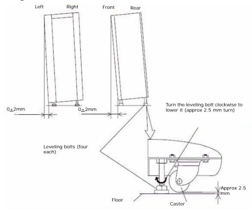
Figure 3-23: Example of Lowering the Leveling Feet
