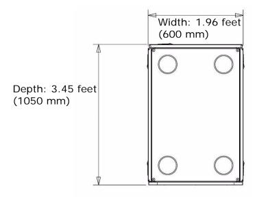
Figure 3-3: Top of the Hitachi AMS 2000 Rack
