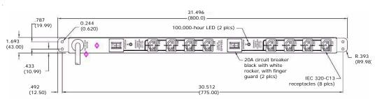
Figure 3-6: Hitachi AMS 2000 Family Rack PDU Design
