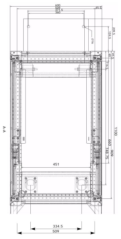
Figure 3-36: Detailed Cross-Section View (EMEA Rack)
