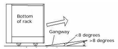
Figure 3-26: Maximum Incline (Slope) for Moving the Rack
