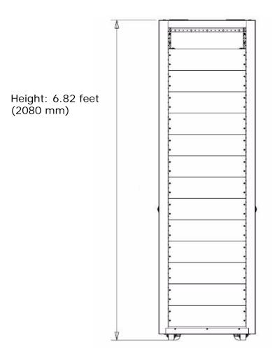
Figure 3-2: Front of the Hitachi AMS 2000 Rack
