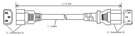
Figure 3-9: Power Jumper Cable (250 VAC 10A IEC320-C14)
