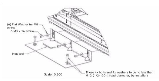
Figure 3-24: Example of Installing the Side Stabilizer Plates (Detail A)
