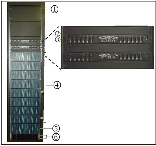
Figure 6-1: AMS 2500 DC-powered Storage System
