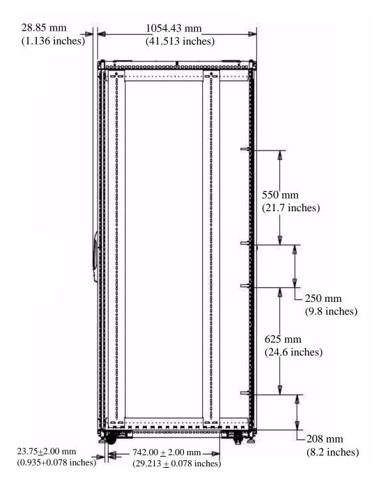
Figure 3-16: Side View of Hitachi AMS 47U Rack
