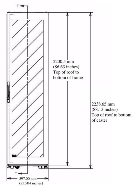
Figure 3-15: Front View of Hitachi AMS 47U Rack
