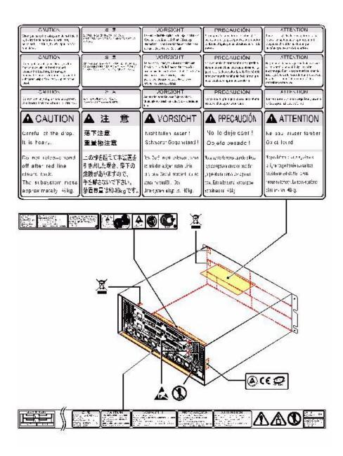
Figure 2-2: Example of Safety Labels on AMS 2500 Base Unit
