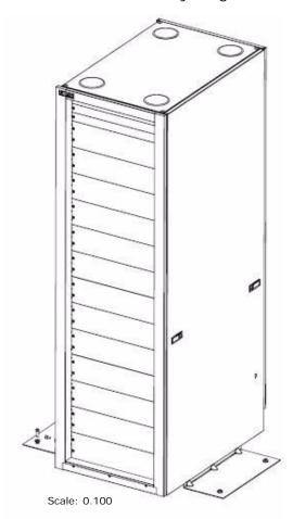
Figure 3-25: View of Hitachi Rack with Side Stabilizer Plates Installed
