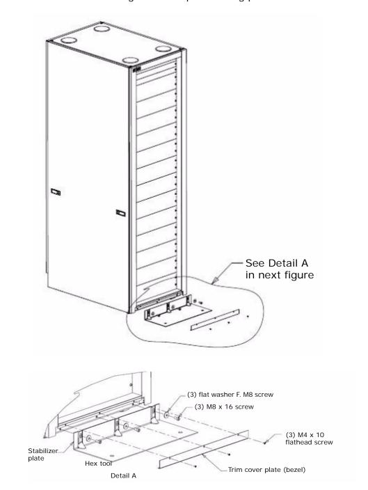
Figure 3-31: Installing and Uninstalling the Anti-Tip Stabilizing Plate
