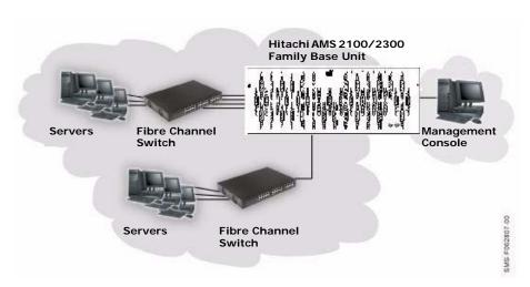
Figure 4-3: Example of a Switch Configuration
