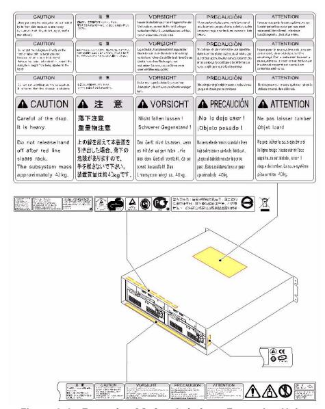
Figure 2-3: Example of Safety Labels on Expansion Unit
