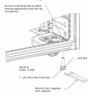
Figure 3-22: Example of Leveling Feet
