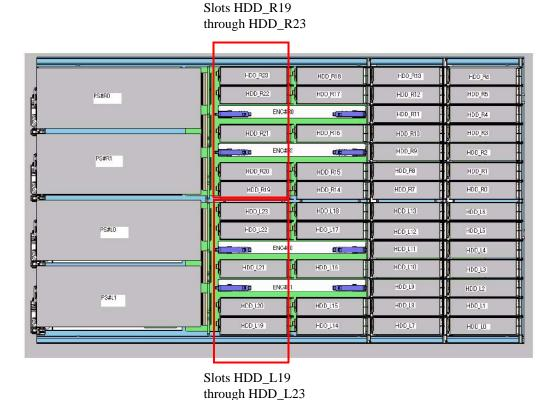
Figure 1-1: AMS High-Density Expansion Unit Drive Slots
