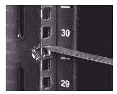
Figure 3-30: Installing the Cage Nuts
