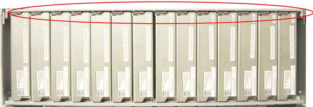
Figure 4-32: Alarm LED Locations
