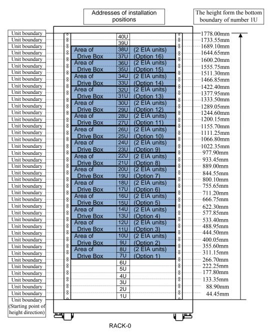
Fig. 3.4.5-2 Whole Layout of Installation Position Addresses (RACK-0)
