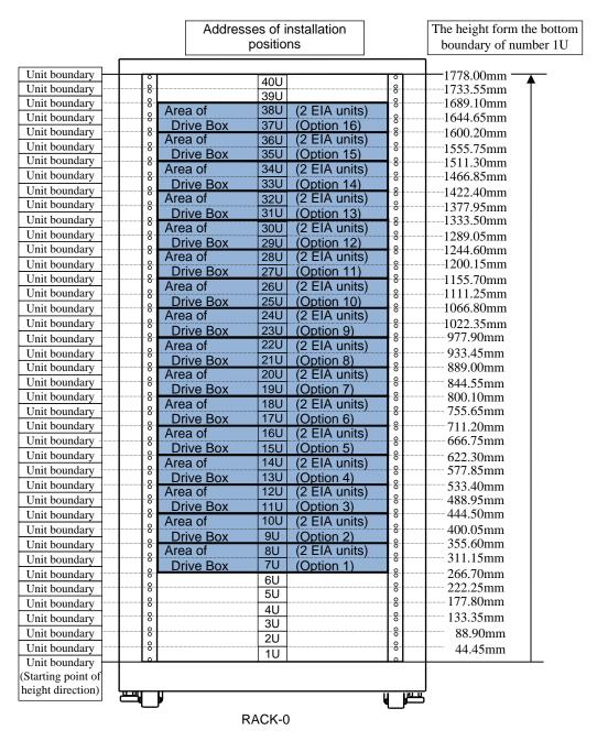
Fig. 4.2-1 Mounting Location of Drive Box
