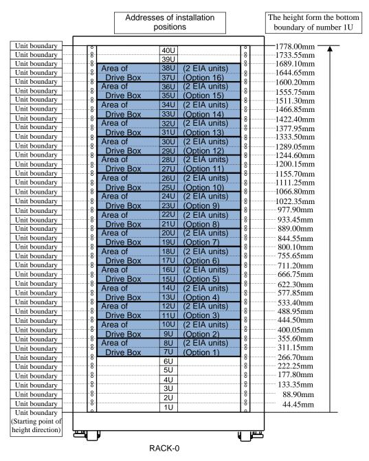
Fig. 3.4.3-2 Whole Layout of Installation Position Addresses (RACK-0)
