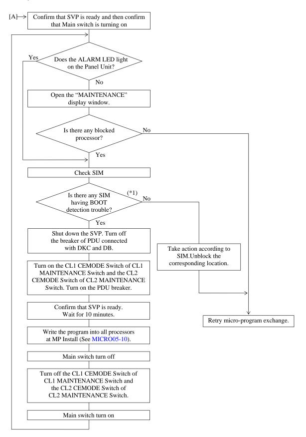
[Recovery Procedure for Communication Time-out/PC Trouble in Downloading Micro-program /Version incompatibility]
