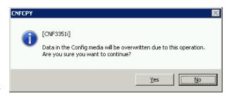
Config media is not necessary, select the [No] button and go back to step (3).
