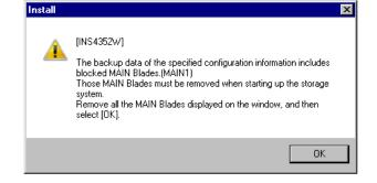
NOTE: When there is not a blocked part in MAIN Blade, this message is not displayed.
