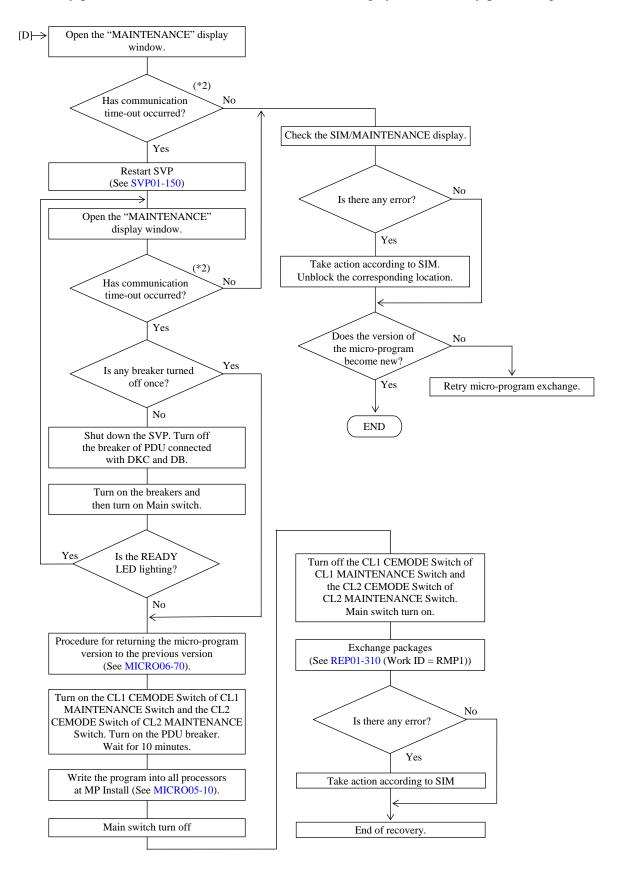
[Recovery Procedure for an error in data transferred to the DKC/AP error/SVP error]
