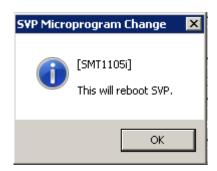
NOTE: After SVP reboot, because the connection with the Clients PC and the SVP goes out, make re-connection (refer to SVP 1.5.2) and check surely the message of the microprogram exchange end.
