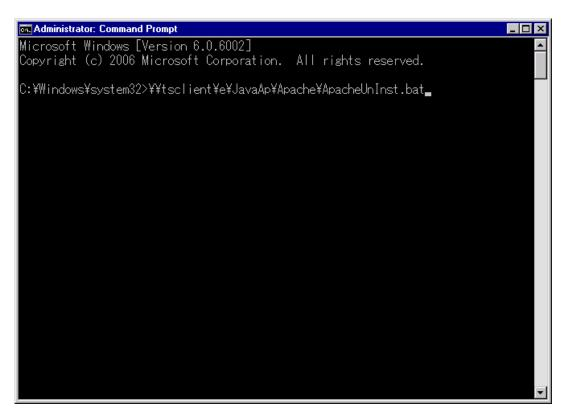
NOTE: After uninstallation of Apache is finished, you MUST next complete the procedure in "4.1.2 Installation of Apache" before modifying any other software product on the SVP.
