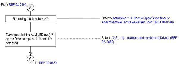
\*1: For the DBX, remove the front bezel, pull the array out of the rack, and remove the top cover. For the DBW, the front bezel does not need to be removed. Pull the drawer out of the array.
