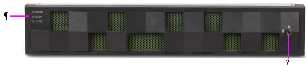
Figure 2-20: DBL/DBLD front panel bezel
