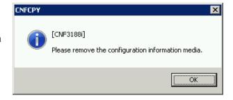
(6) Select (CL) [Exit] of the 'Copy Config Files', and execute 'Define Configuration & Install' (go to INST05-80).
