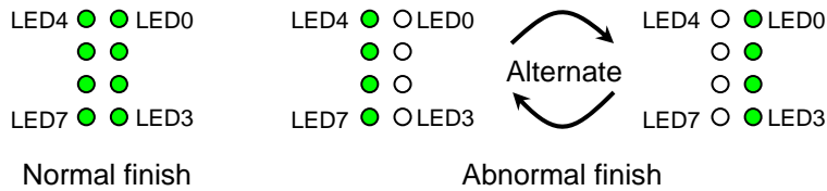
Fig. 3.2.6.1.1-4 Status LED's condition after the recovery process
