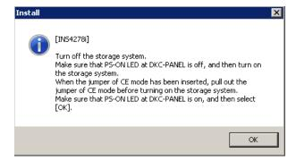
NOTE: Pull out the CEMD jumper from MPB when powering on the storage system in CE mode by the CE mode switch.
