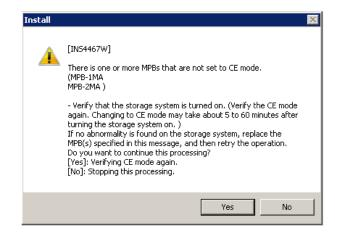
NOTE: The time required to change to CE mode after turning the storage system ON varies depending on cache size. When a cache PCB with the maximum size (524,288 MB) is mounted, changing to CE mode may take up to 60 minutes.
