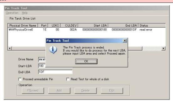
When the status is changed to "read error" and the device remains in the list, go to Subsection TRBL05-530, "Operation of Unreadable Pin Process".
