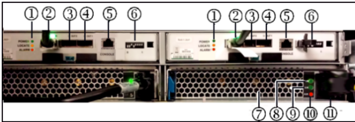
Figure 1-12 2U SFF and LFF drive tray, rear view
