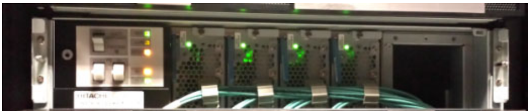
Figure 5-1 VSP G1000 controller upper panel
