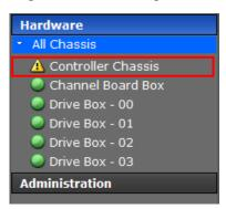
(2) <Controller Chassis window> Click the [CTLs] tab in the "Controller Chassis" window to display a Controller Board status. See MAINTENANCE PC SECTION "3.22 Alert Display Related to FRU (Field Replacement Unit)" for the [Status].
