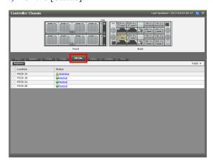
(3) <Select PCIe Channel Board> Select a PCIe Channel Board to be replaced. Click the [Replace] button.
