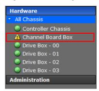
(2) <Channel Board Box window> Click the [FANs] tab in the "Channel Board Box" window to display a CHBBFAN status. See MAINTENANCE PC SECTION "3.22 Alert Display Related to FRU (Field Replacement Unit)" for the [Status].
