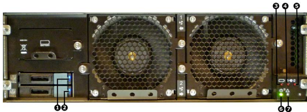
Figure 7 Models 4060, 4080, and 4100 status LEDs
