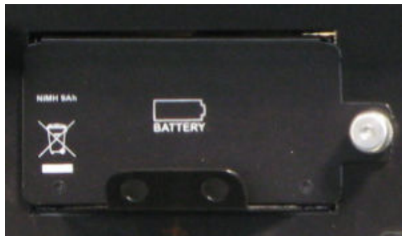
Figure 9 Model 4060, 4080, and 4100 NVRAM backup battery pack (front view)
