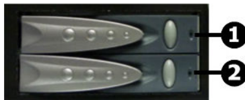
Figure 10 Hard disk drives status and activity status LEDs - model 4040
