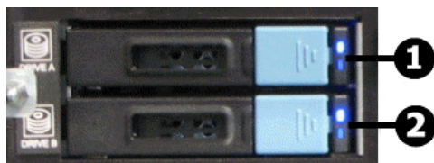
Figure 11 Hard disk drives status and activity status LEDs - models 4060, 4080, and 4100
