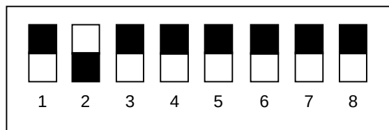
Figure 5.2.4 DIP Switch Setting for Memory Dump
