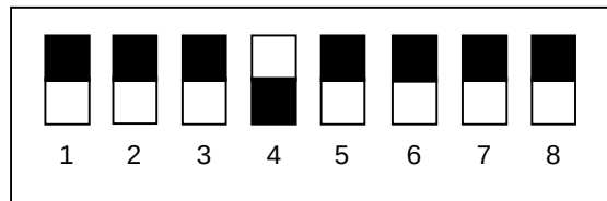
Figure 4.1 DIP Switch Settings for Download Program
