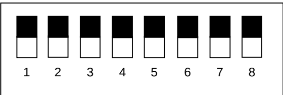
Figure 5.1.2 DIP Switch, shifting to Dual System has not started yet.
