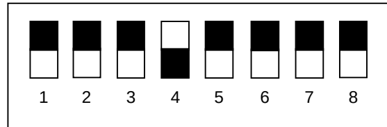
Figure 6.11.1 DIP Switches (Being set for System parameter settings)
